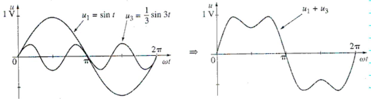
Figure 10.12. Recombination of the rectangular signal with the fundamental and the 3rd harmonic
