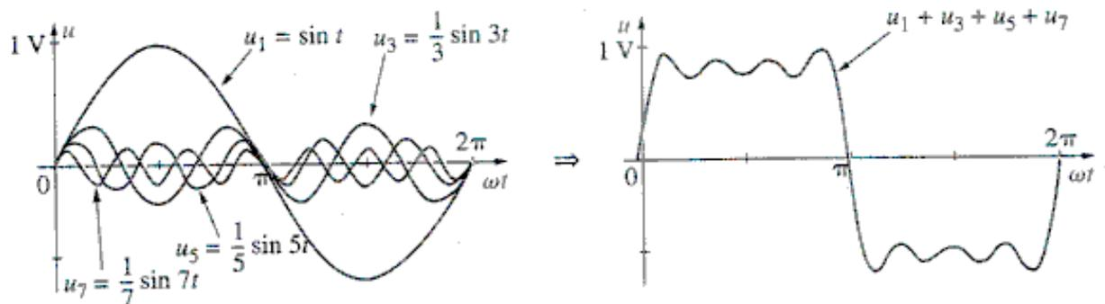
Figure 10.13. Effect of adding the 5th and 7th harmonics
